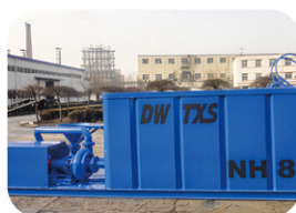
Mud mixing unit
