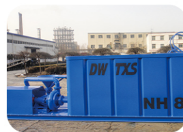
Mud mixing unit
