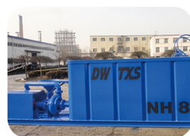
Mud mixing unit
