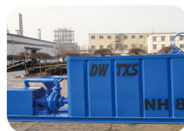
Mud mixing unit
