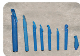
Beacon housing and drill bit
