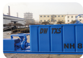
Mud mixing unit
