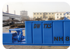
Mud mixing unit
