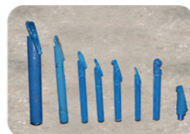
Beacon housing and drill bit
