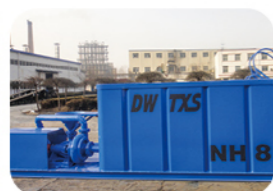
Mud mixing unit
