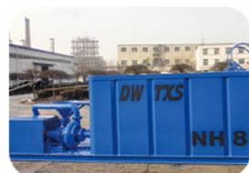
Mud mixing unit
