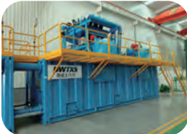
Mud mixing & recycling
